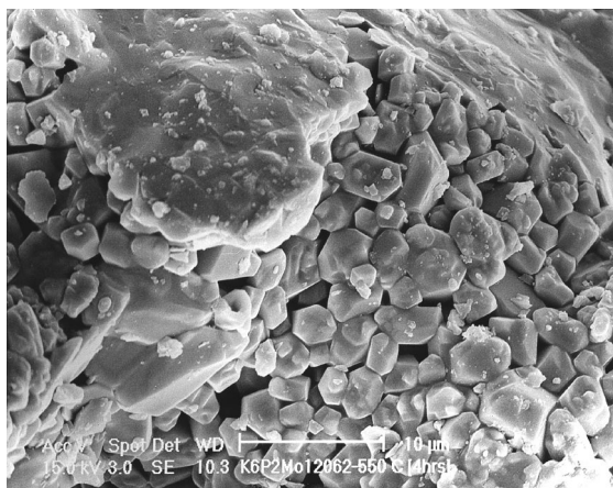
Fig. 7. SEM image of K_6[P_2Mo_{18}O_{62}] \cdot 4C_4H_8O_2 \cdot 16H_2O after thermal treatment and rearrangement at 550^\circ\text{C} for 4 h in air.
